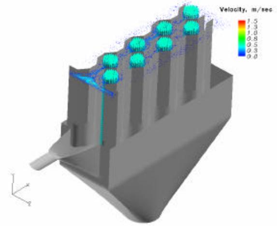
**Figure 11. CFD Simulation. Center Plane Gas Flow Distribution. Top View**
