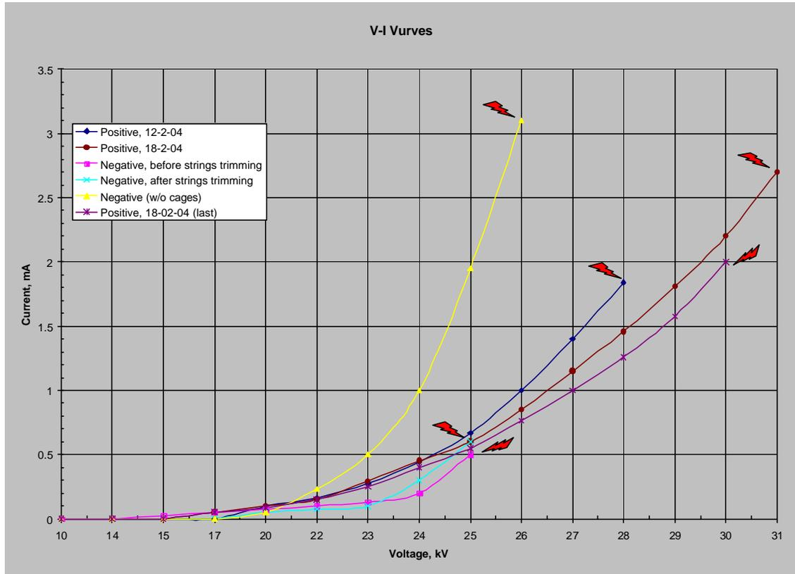
A high-voltage power supply with the ability to provide both positive and negative voltage was utilized to charge the corrugated plates. The goals of these shake-down tests were two-fold. The first was to evaluate the electrical clearances in the pilot-scale unit and to identify any plate/electrode/BFE alignment issues that would result in premature “back corona” or sparking. Once any alignment issues were identified and corrected, the V-I response of the unit was fully characterized.
