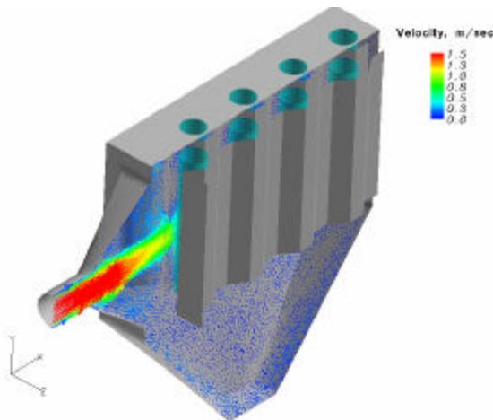
The model included MSC inlet, filtration bags and internal electrodes. The gas flow properties for CFD model were based on the data from Table 1. The simulation was based on ideal gas with air properties; two parameters  $\epsilon$  turbulence model was employed with smooth wall boundary condition on MSC™ wall and internal electrodes and barriers.
