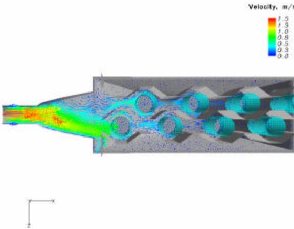
**Figure 12. CFD Simulation. Bags Exit Gas Flow. Top View**
