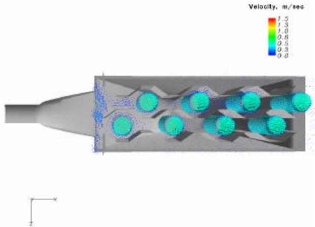
The model included MSC inlet, filtration bags and internal electrodes.
