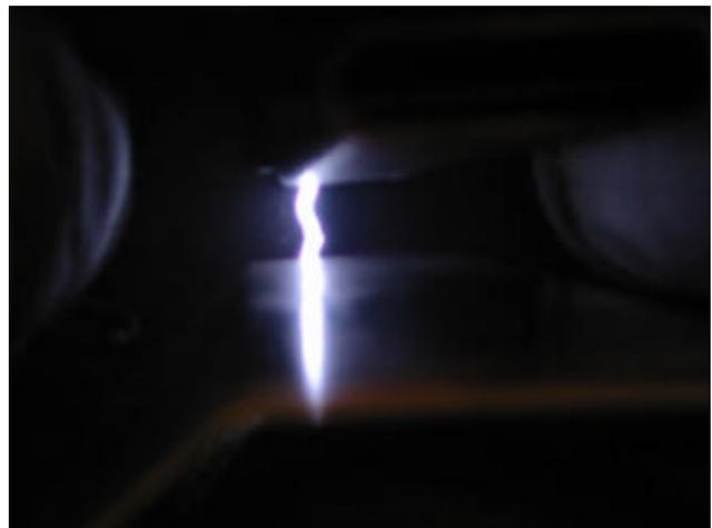
Figure 13 presents the results of the initial V-I characterization of the pilot MSC. The initial tests on 2/12/04 were run in the positive corona mode, and the maximum voltage attainable prior to the onset of sparking was 28 kV. These initial tests were run with the hopper, inlet and all inspection panels
